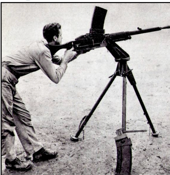
Model 93 (1933) 13-mm heavy MG Caliber..... 0.519 inch Principle of operation..... Gas-operated, full-automatic only Ammunition..... Ball, tracer, and armor-piercing Total weight of each gun..... 87 pounds Muzzle velocity: Ball ammunition..... 2,210 feet per second Armor-piercing ammunition..... 2,280 feet per second
