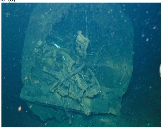
52 feet of bow is missing. Note crimping
