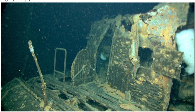
The fairwater free flooding area just in front of the conning tower
