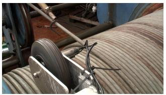
This mechanism moves back and forth making the cable lie level. It failed and cable spilled off the spool and jammed. It was late at night and it meant that the towfish could not be pulled in, a very serious situation
