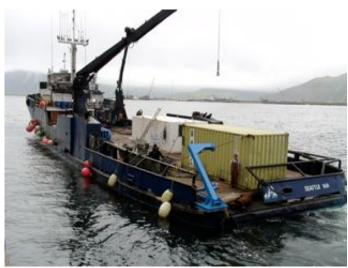
The *Aquila*, originally a 1972 oil rig supply boat converted for crab fishing.
