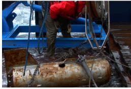
1500 lb. depressor that holds towfish down and helps keep towfish movement steady
